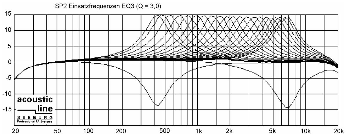
Fig. 11 Measured frequency response curves for EQ3
