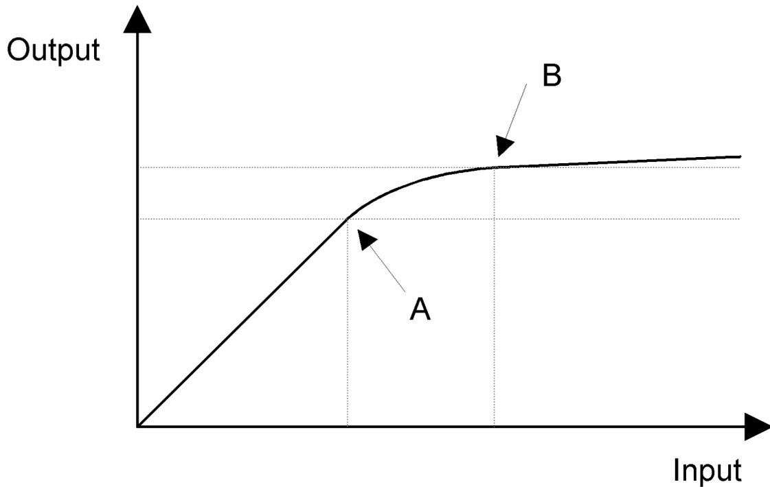
**Fig. 8** Characteristic curve of the SP2 limiter. The limit indicator LED lights up at point A. The compression ratio increases with an increasing input signal (area between A and B). The maximum compression ratio of 1:20 is reached beyond B.
