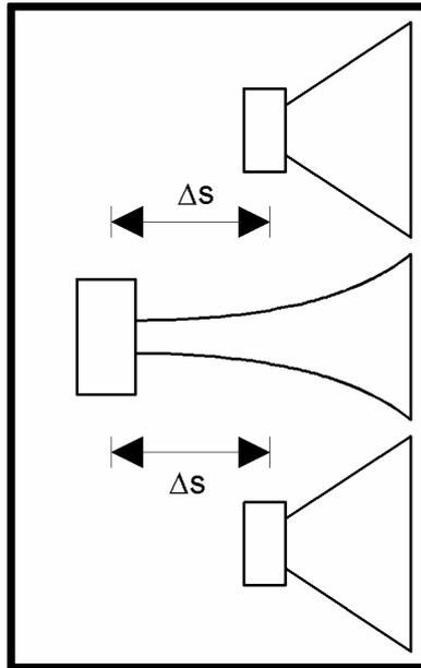
**Fig. 6** Displaced Speakers
