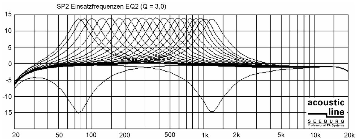
Fig. 10 Measured frequency response curves for EQ2
