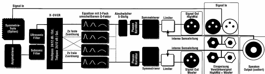
**Fig. 2** Block diagram of the SP2
