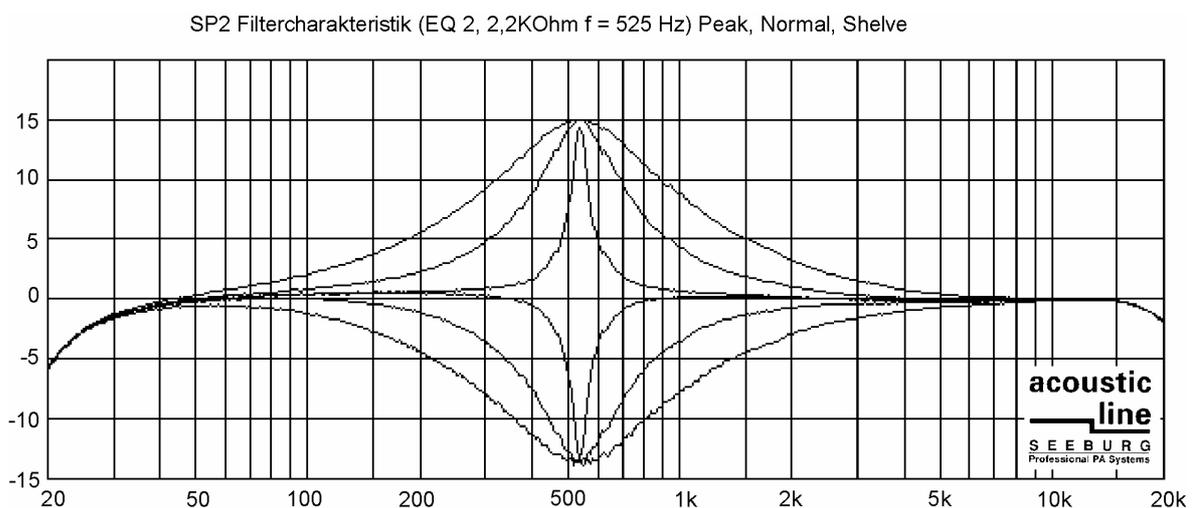
**Fig. 13** Characteristic curves of the EQ filters with three different Q factors preset.
