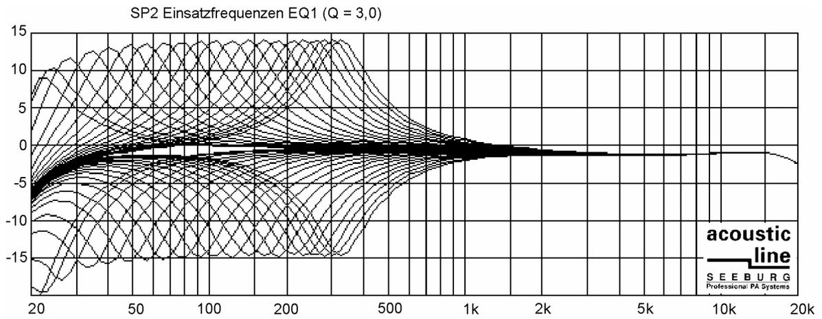
Fig. 9 Measured frequency response curves for EQ1
