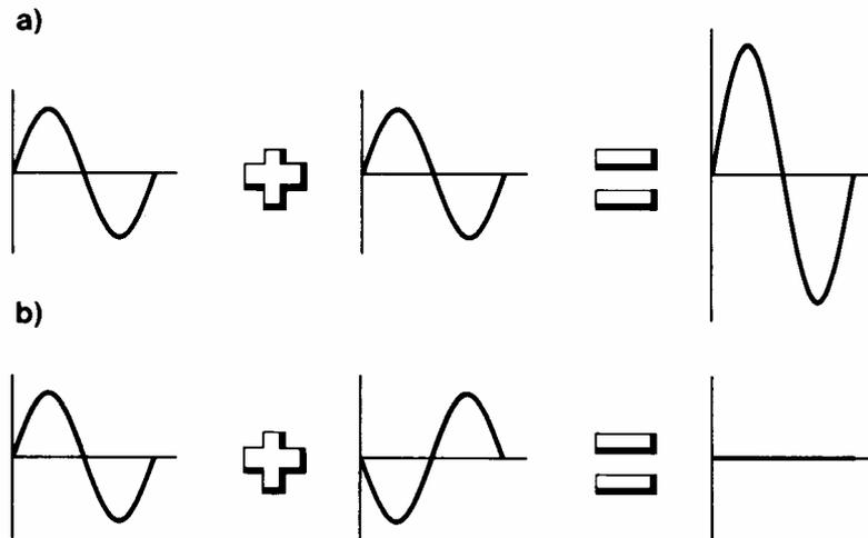
**Fig. 16** Two waves of equal amplitude, frequency and phase add up to a wave of twice the amplitude (a).
