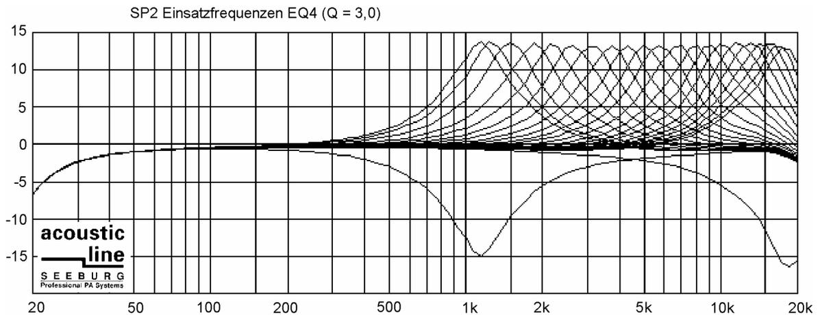
**Fig. 12** Measured frequency response curves for EQ4
