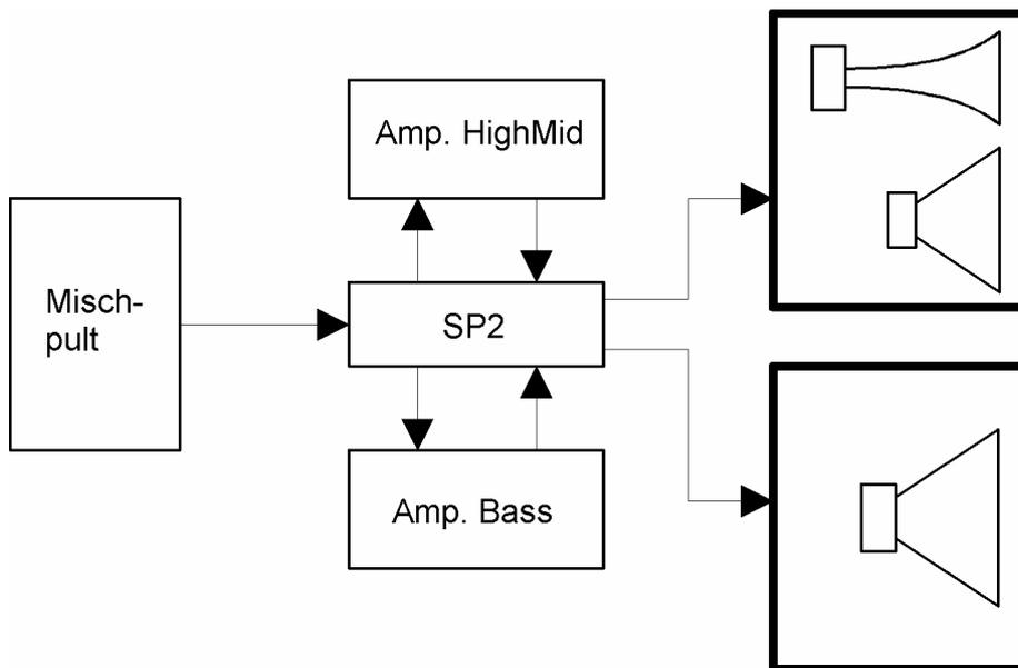
**Fig. 1** How the SP2 is hooked up (only one channel pictured).
