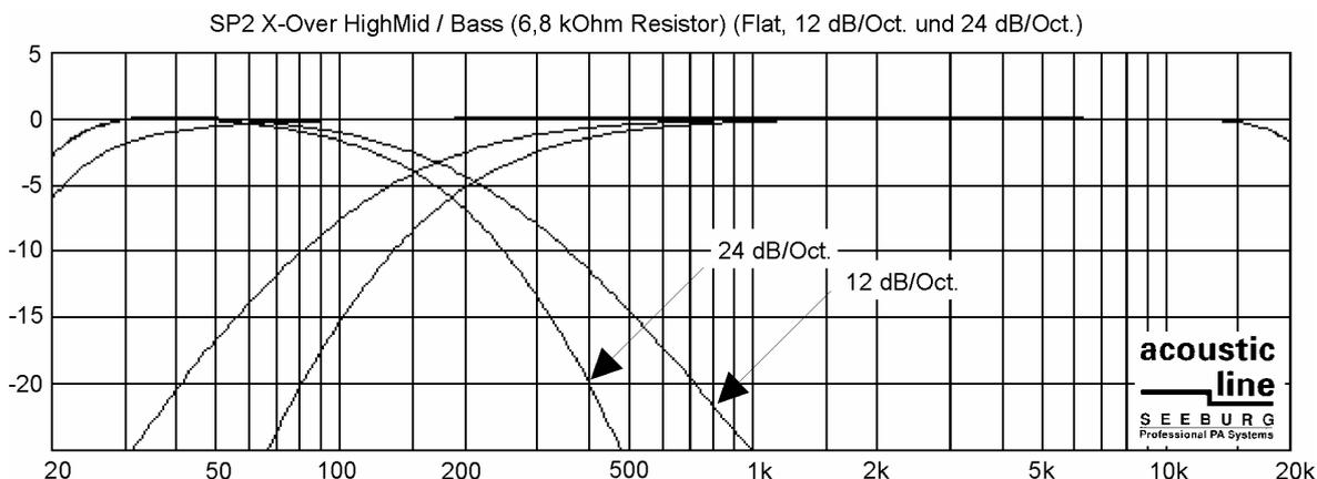
**Fig. 5** Measured frequency responses of the SP2 frequency dividing network.
