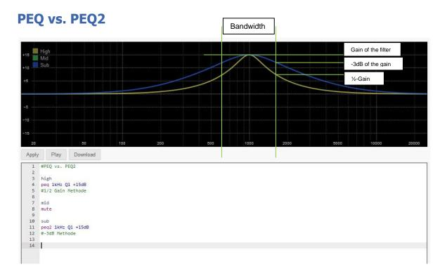
For the same gain and quality factor, the filter calculated according to PEQ2 is wider than the filter calculated according to PEQ. The resulting frequency response curve always depends on the gain and on the quality factor of the filter.
