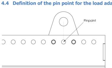
The load adapter for connecting the Flying Frame to a chain hoist or winch is constructed symmetrically to prevent confusion. The pin point calculated by the simulation software EASE Focus 3 is always the empty hole between the two Locking Pins used to secure the load adapter. This hole is consequently always directly below the shackle in the load adapter.
