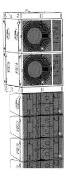
It's possible to mount Galeo T units under flown Galeo T Subs by using a further Galeo T Flying Frame that's mounted under the lowest Galeo T Sub. The maximum number of flown subwoofers and Galeo T units can be found in the description in section 5.1. For the flown Galeo T Subs it is recommended to use the same controller setup as for the ones on the ground.
