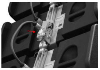
Checking that all of the Auto-Locking Hooks have locked in correctly
