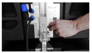
Frame, always has a splay angle of 0° for mechanical reasons.
