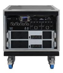
The 7U standard system rack offers 8x inputs (4x analog and AES, 8x DANTE optional) and 8x amplifier outputs for the speakers. The heart of the system is the HDLM 8 system controller, which is responsible for the entire speaker processing. All connections required for the system are located on the front of the CP 4.8. connection panel and can therefore be reached quickly by the user. On the rear of the CP 4.8 there is also the three-phase power distribution with the CEE 16 A connector.
