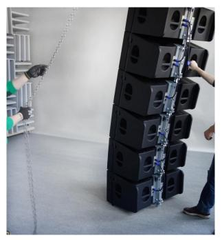
Setting the curve of the Galeo T Arrays by placing the arrays on the floor
