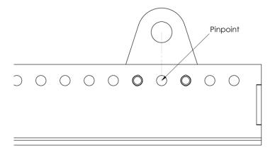
The load adapter for connecting the Flying Frame to a chain hoist or winch is constructed symmetrically to prevent confusion. The pin point calculated by the simulation software EASE Focus 3 is always the empty hole between the two Locking Pins used to secure the load adapter. This hole is consequently always directly below the shackle in the load adapter.
